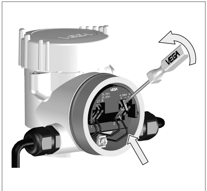
Fig. 14: Connection steps 5 and 6
