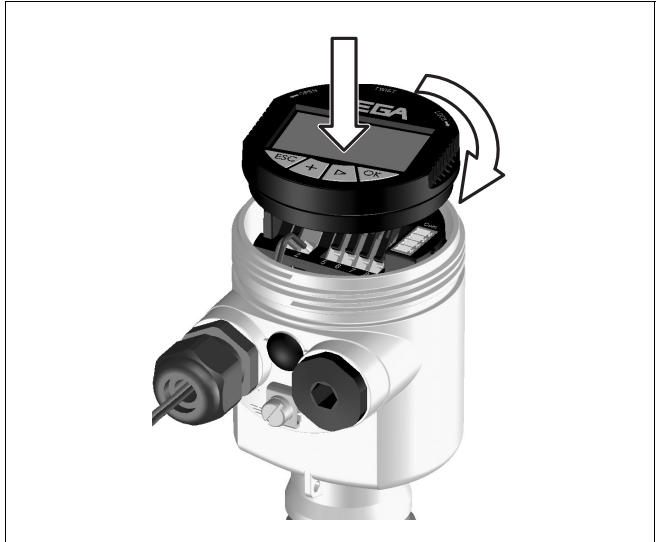
Fig. 16: Installation of PLICSCOM
