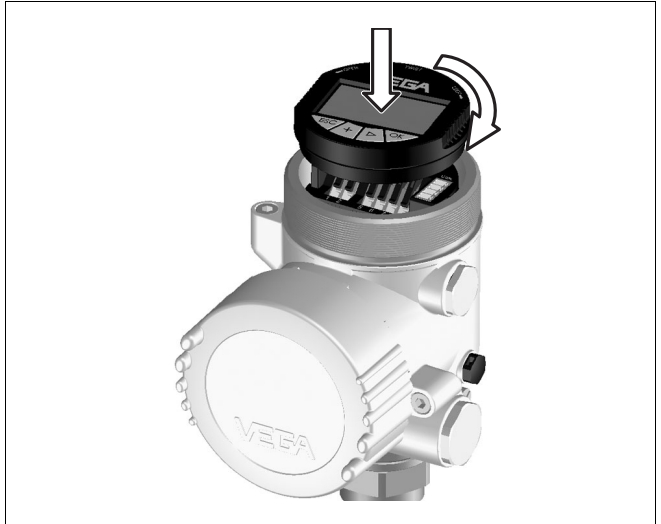
Fig. 16: Installation of PLICSCOM
