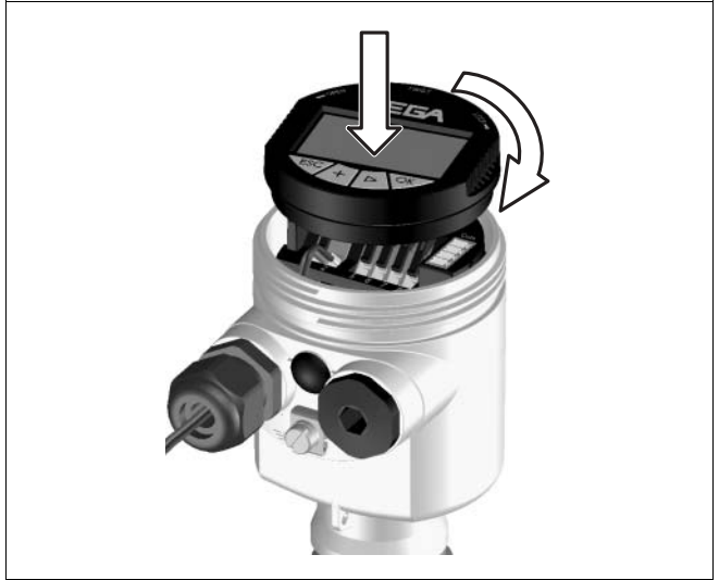
Fig. 26: Installation of PLICSCOM
